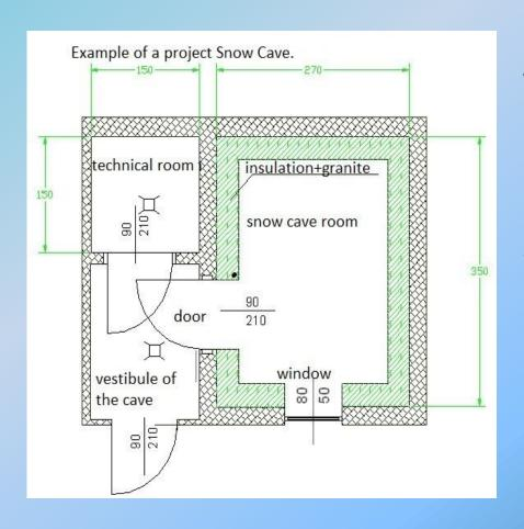
The minimum dimensions of the cave is a 3 m  $\times$  3 m. Snowmaking nozzle is located beneath the ceiling, which, with a spacious room gives a great visual effect. Additionally, in front of the entrance to the cave there should be a vestibule in order to limit the loss of chill from the cave and lessen the thermal shock.
